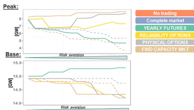
Fig. 12. Impact of the forward capacity market on the peak and the base capacities as function of risk aversion.
